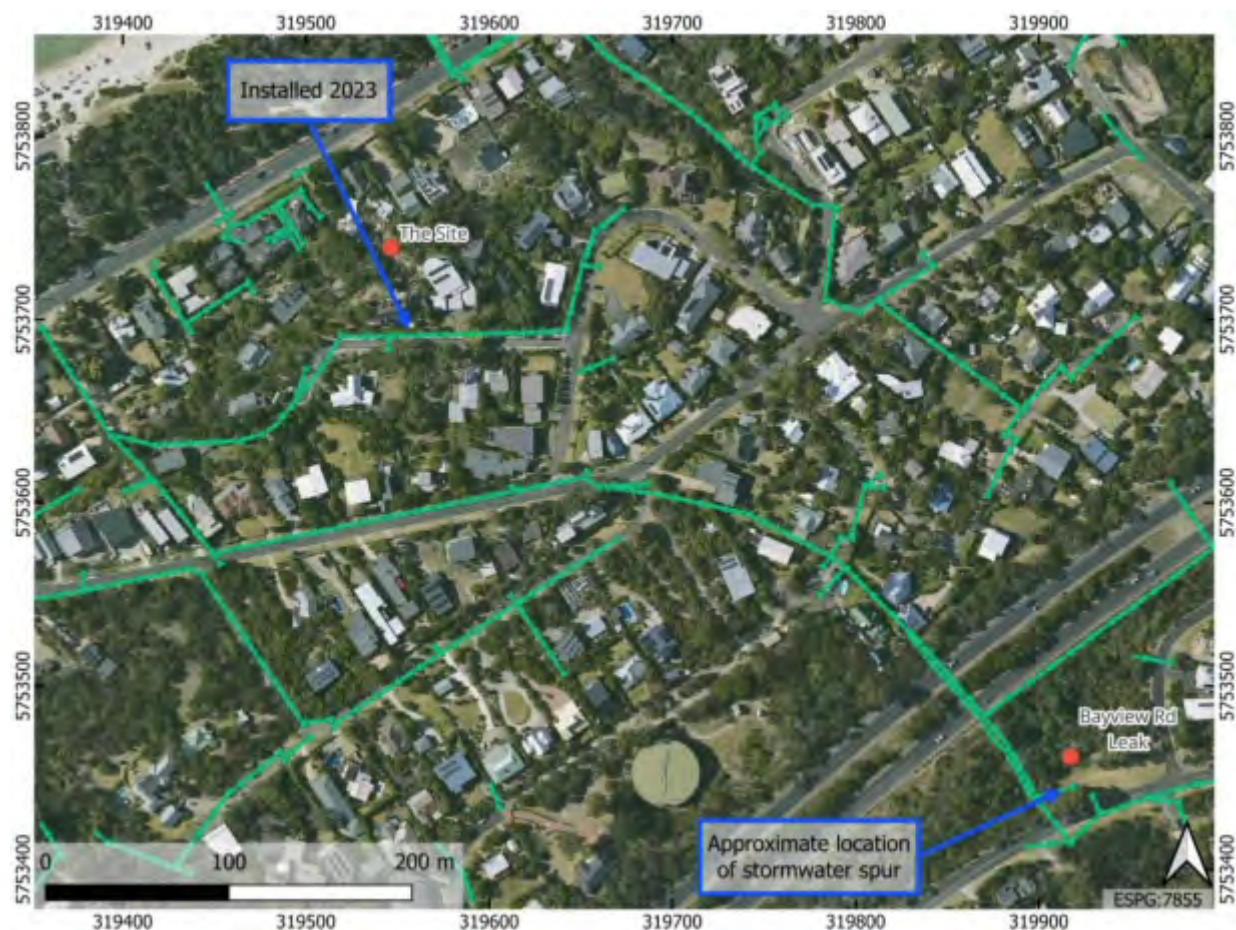
Figure 21: Map (not scaled) showing stormwater drainage network in the locality of the Site. Annotations have been added by SMEC of the stormwater drainage constructed in 2023 and known ‘spur’ confirmed by MPSC
