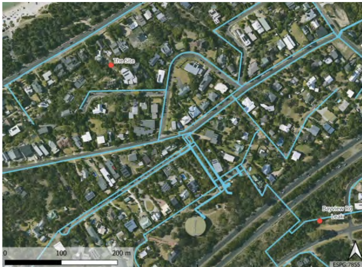
Figure 18: Plan showing water mains network (blue) around the locality of View Point Road
