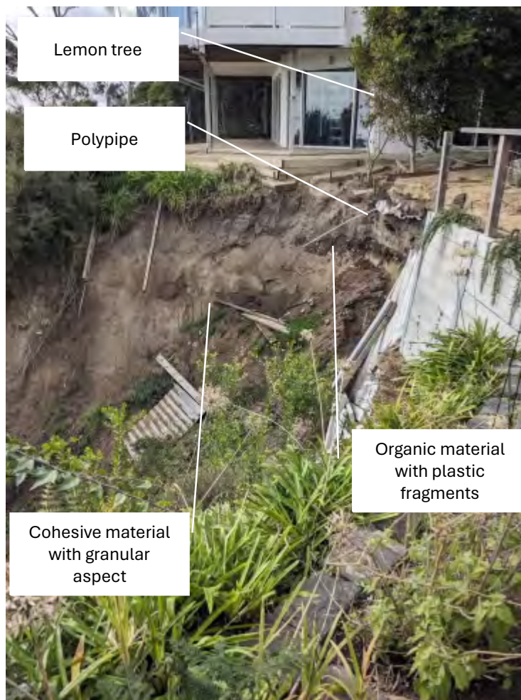
Figure 4: 17/6/25 Photo 01 Looking east showing the detail of the backscarp. Note the vertical nature of the backscarp, approximately 4.5m high.
