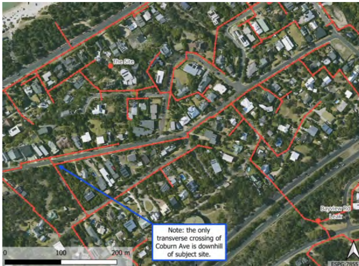
Figure 17: Plan showing sewerage network (red) around locality of View Point Road. Note that the leak near Bayview Road is on the south side of Mornington Freeway.
