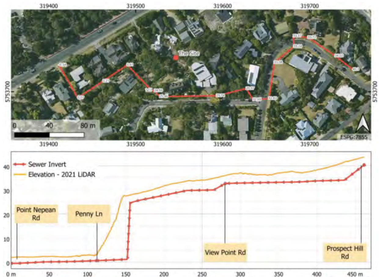
Figure 20: Graphical long section showing the ground level (CL) and invert levels (IL) of the sewer network between Prospect Hill Road and Point Nepean Road.
