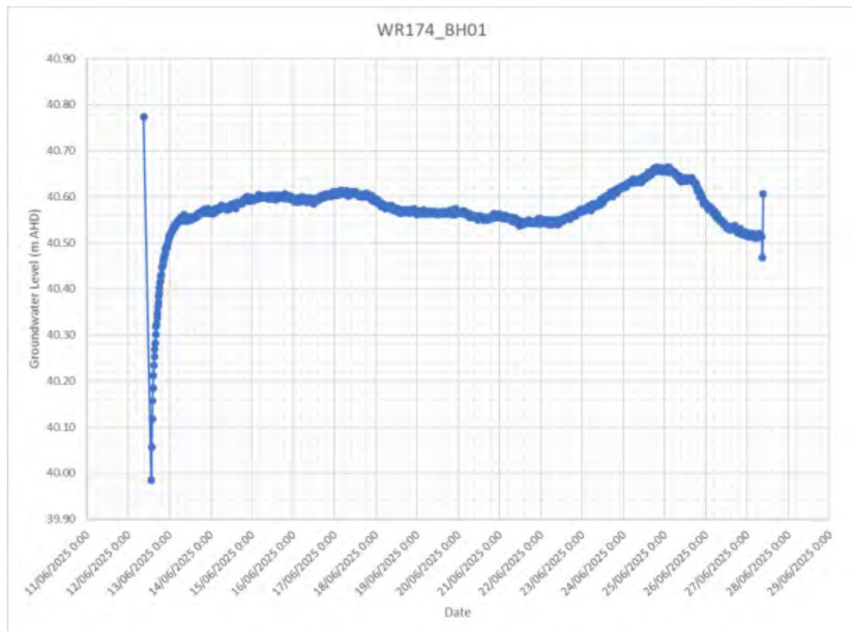
Figure 5: WR174_BH01 groundwater level readings
