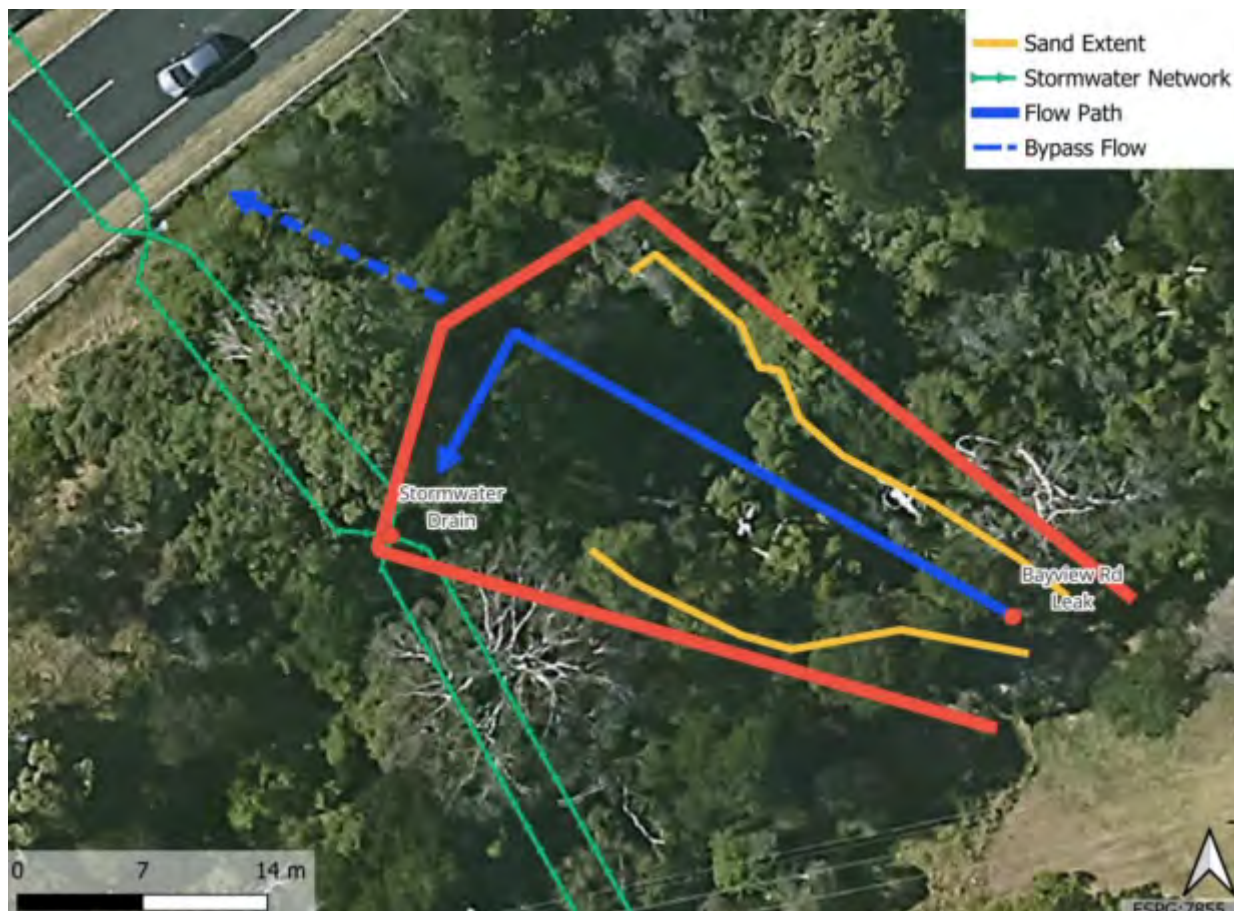
Figure 34: Schematic model of the Bayview Road leak showing surface extents and possible flow paths
