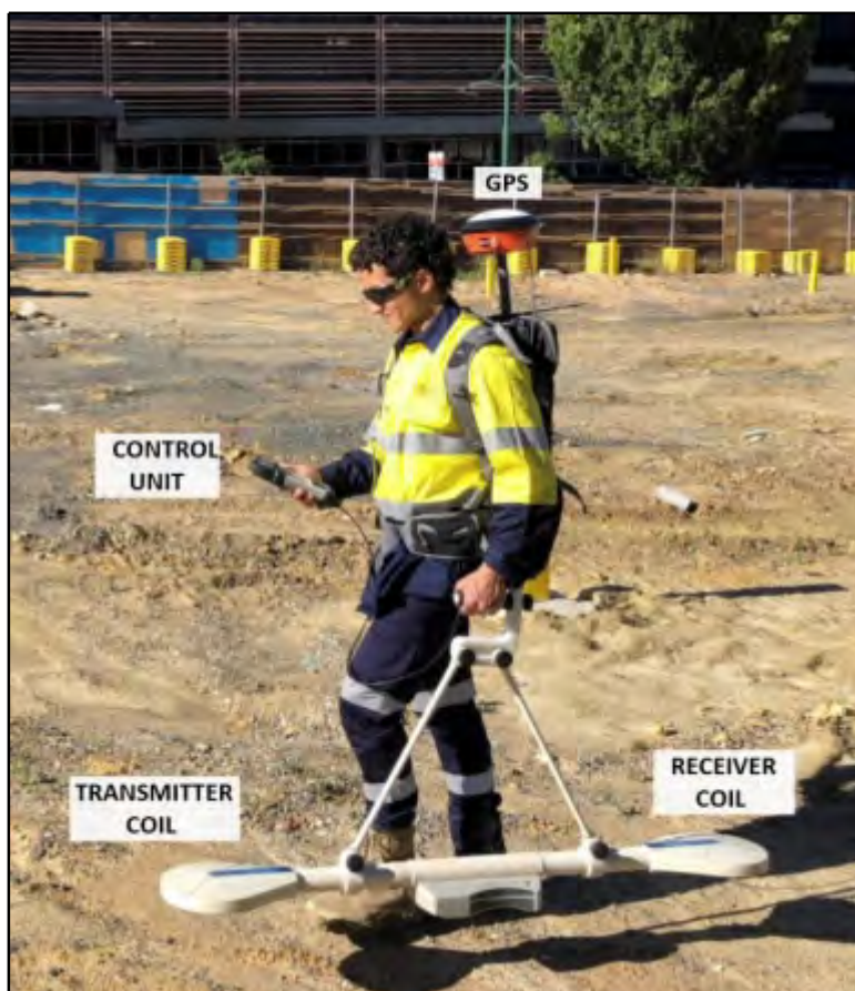
Figure 1: FEM collection using the GSSI Profiler EM400 during a similar survey
