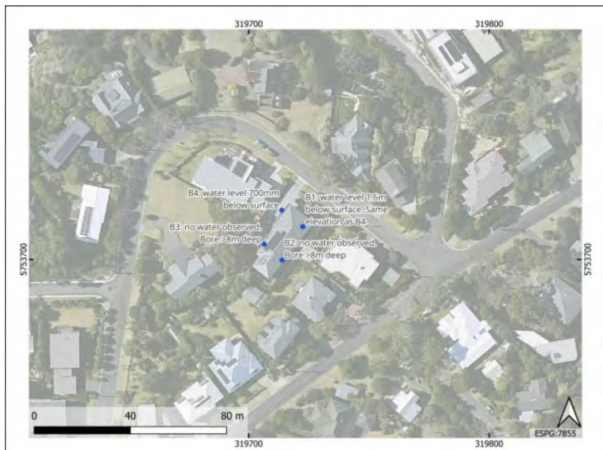
Figure 28: Locations of boreholes drilled in 2018 prior to the construction of No. 5 Prospect Hill Road, noting water level observations.
